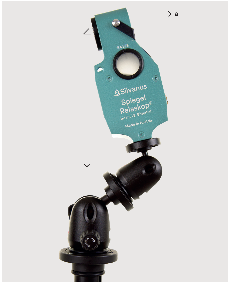
Fig. 4: The Spiegel Relaskop mounted on a tripod with lockable ball joints a – horizontal distance from the eye to the center of the tree Cross-section
