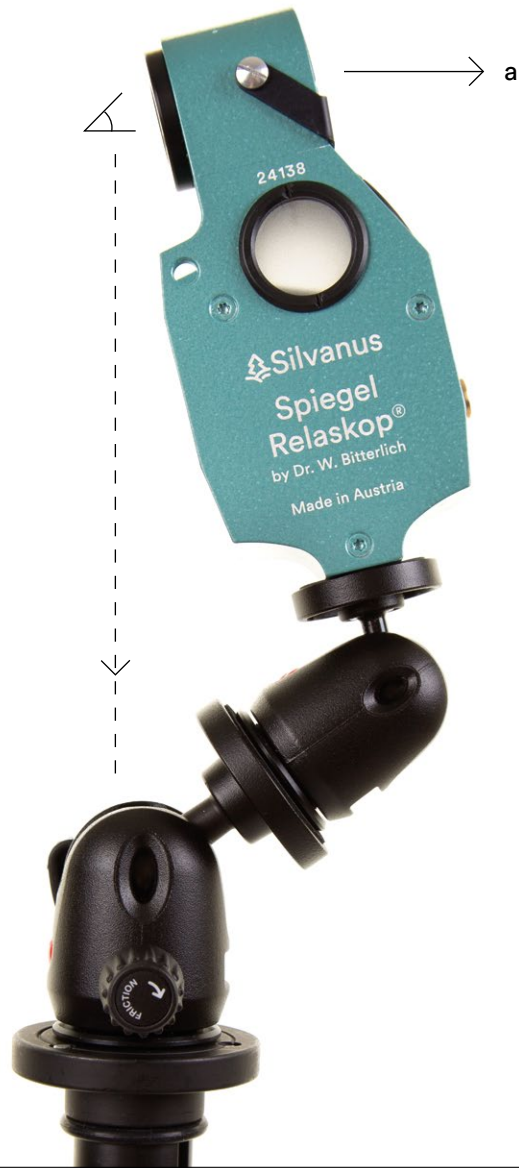
Fig. 2: The Spiegel Relaskop mounted on a tripod with lockable ball joints
